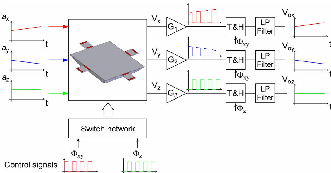
Figure 4. Block diagram of the interface circuit.
