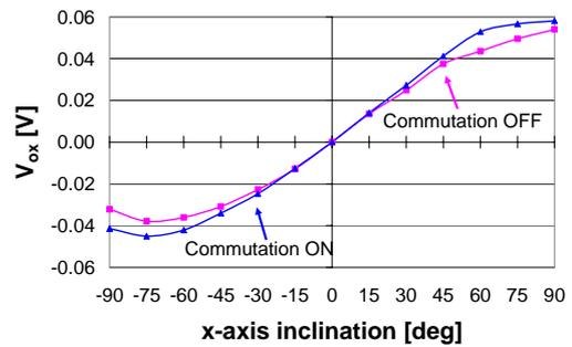
Figure 6.  $V_{ox}$  circuit output versus  $x$ -axis static inclination.
