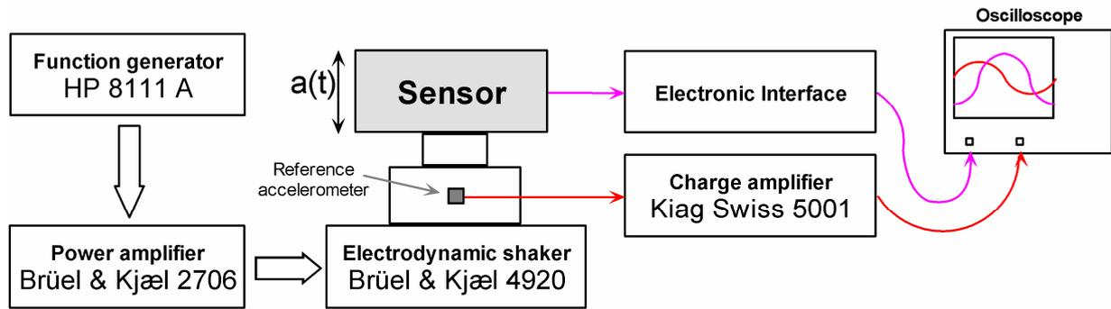
Figure 9. Experimental setup for the dynamic characterization.
