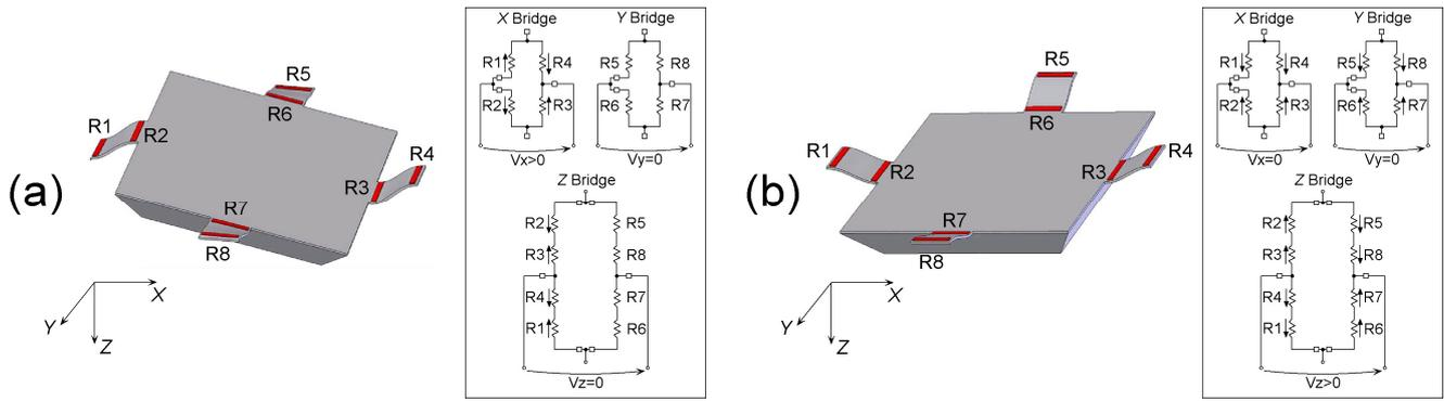
Figure 3. Displacement of the seismic mass and unbalance voltage of the bridges for applied accelerations along the x axis (a) and the z axis (b). The square dots denote the external accessible pads.
