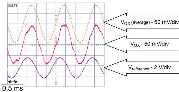
Figure 10.  $V_{ox}$  circuit output for sinusoidal acceleration along x-axis.
