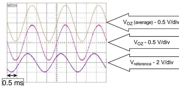
Figure 11.  $V_{oz}$  circuit output for sinusoidal acceleration along z-axis.
