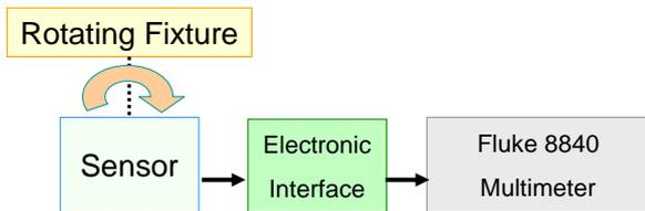
Figure 5. Schematic diagram of the measurement system used for static inclination tests.
