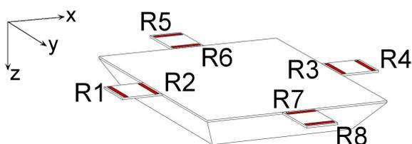
Figure 1. Schematic diagram of the accelerometer structure.
