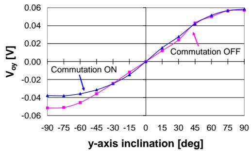
Figure 7.  $V_{oy}$  circuit output versus  $y$ -axis static inclination.
