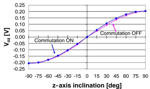
Figure 8.  $V_{oz}$  circuit output versus  $z$ -axis static inclination.
